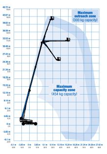
The metric equivalent of working height adds 2 m to platform height. U.S. adds 6 ft to platform height.
