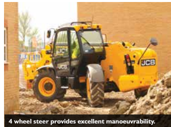
4 wheel steer provides excellent manoeuvrability.
