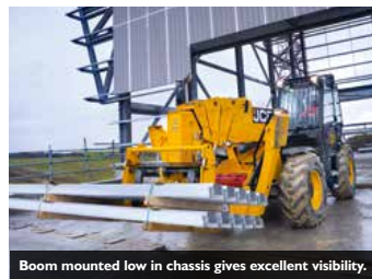
Boom mounted low in chassis gives excellent visibility.
