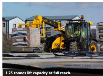
1.25 tonnes lift capacity at full reach.
