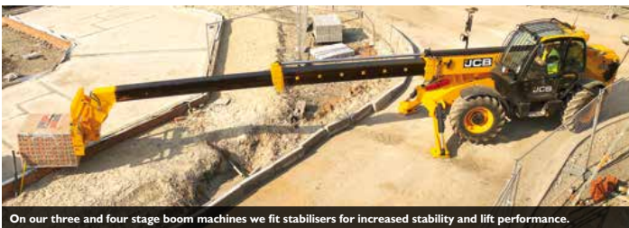
On our three and four stage boom machines we fit stabilisers for increased stability and lift performance.
