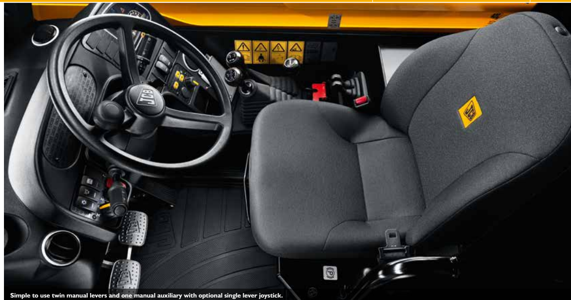
Simple to use twin manual levers and one manual auxiliary with optional single lever joystick.
