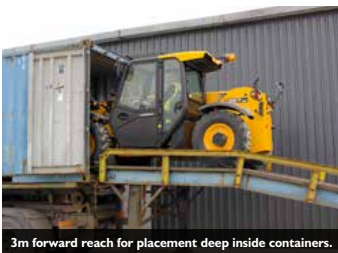
3m forward reach for placement deep inside containers.
