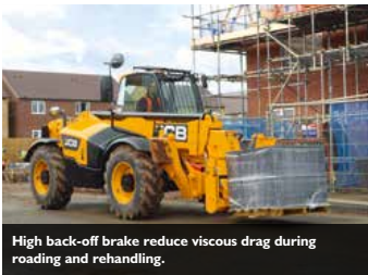
4 wheel steer provides excellent manoeuvrability.
