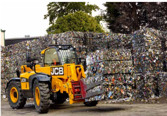
Best-in-class comfort with one of the largest cabs in the industry. The cab conforms to ROPS ISO 3471 and FOPS ISO 3449 and puts the operator firmly in control.
