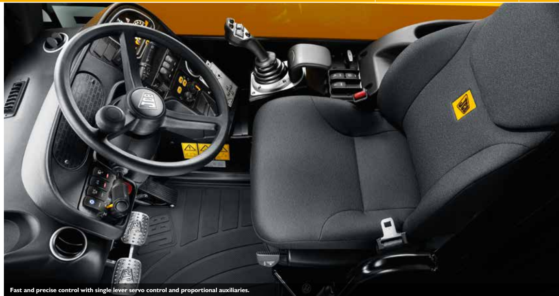
Fast and precise control with single lever servo control and proportional auxiliaries.
