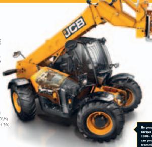
By producing high levels of power and torque even at engine speeds as low as 1300–1400rpm, the EcoMAX engine an provide fuel-efficient matching of transmission and hydraulics.
