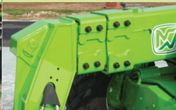
Boom sections slide on adjustable low-friction pads.
