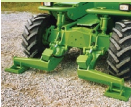
The front stabilisers assure the necessary stability for working on any terrain.
