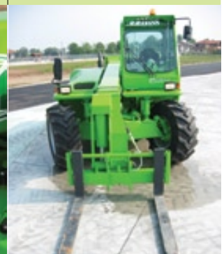
The 'disappearing' boom ensures an excellent 360° visibility.
