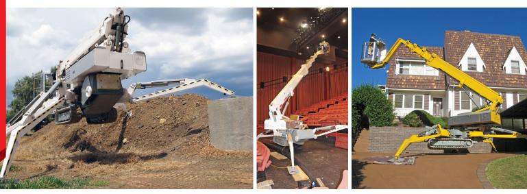
With features including dual power, auto-level, adjustable fly-jib etc, the 23 m Omme Spider Lift weighs only 3250 kg, making it the perfect machine for loadsensitive flooring. The soft non-marking rubber tracks are very gentle on fragile surfaces.
