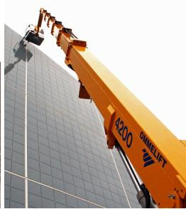
The top of the range Omme 4200 has a huge 42 m working height and a horizontal outreach of 15 m providing an enormous working envelope. And with a weight of only 6.9 t, this Spider Lift is ideal for operating in tight access locations or on load sensitive flooring. The strong all-steel boom sections provide a stable and comfortable platform even at 42 m off the ground!
