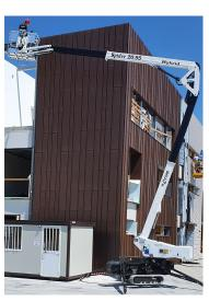
The newly released 2095 is the best performing Spider Lift that weighs under 3.5 t including a trailer. This means that this machine could be towed behind most tradesmen's vehicles.
