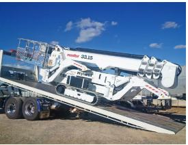
The 3315's unique telescoping articulated boom design provides exceptional up and over outreach specifications. Dual position stabiliser legs allow the 3315 to be set-up in the most difficult locations. Even with the stabilisers set in the narrow position, a complete 360 degrees slew is still possible!
