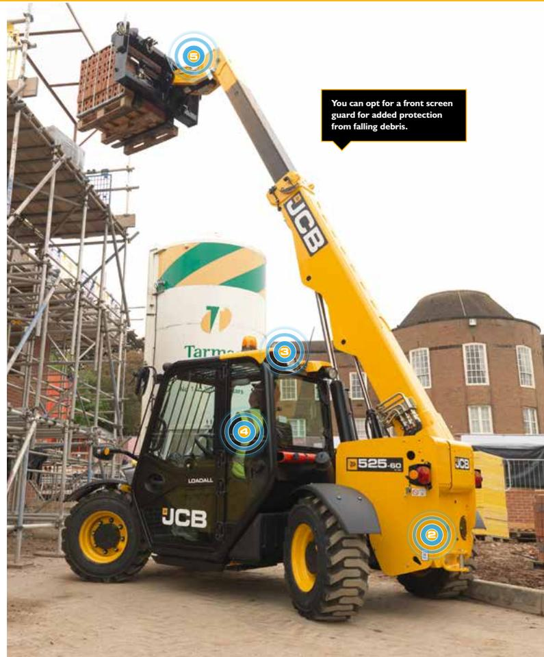
The 525-60 Hi Viz Loadall is equipped with a full set of side mirrors for excellent visibility and full safety compliance.
