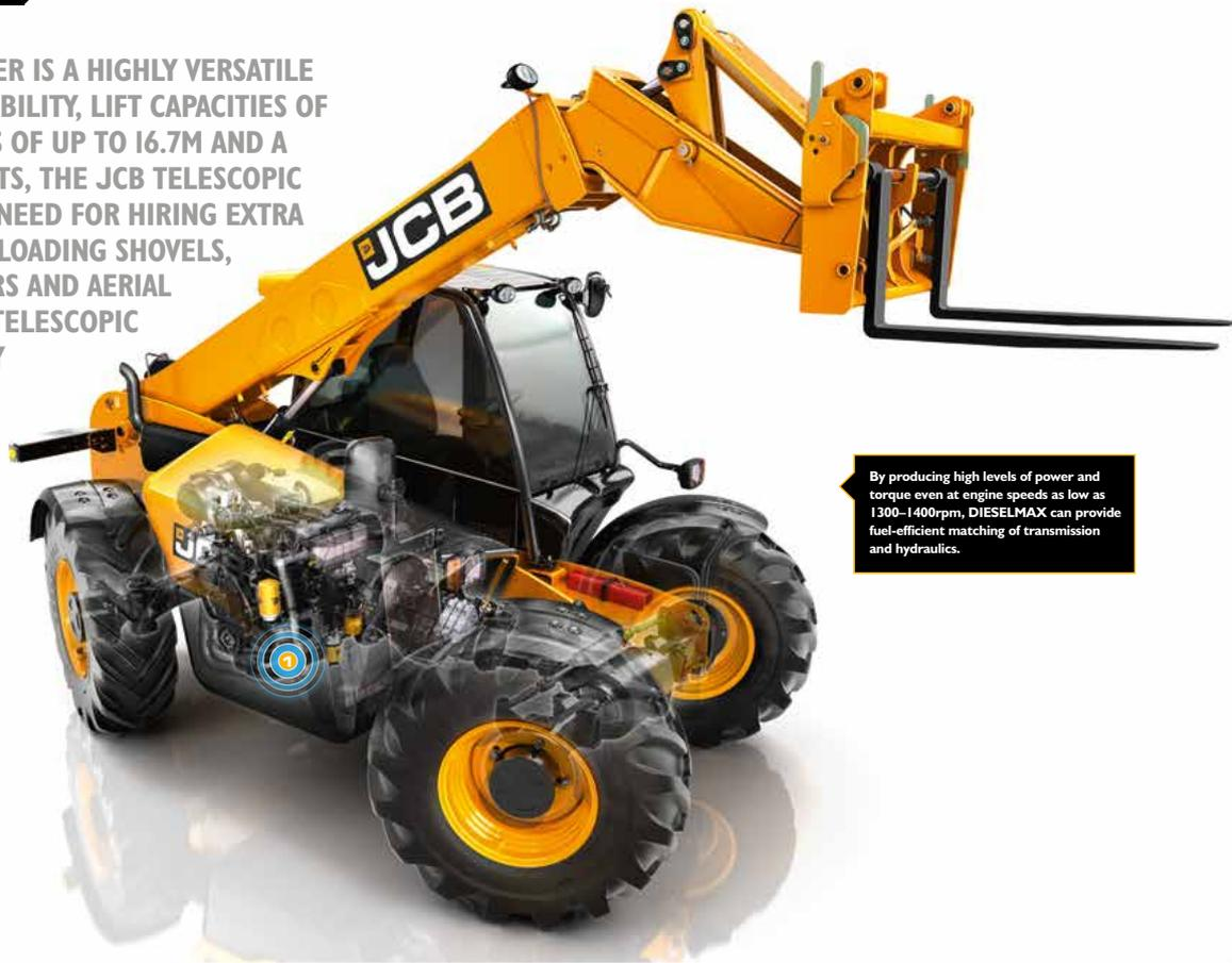
By producing high levels of power and torque even at engine speeds as low as 1300-1400rpm, DIESELMAX can provide fuel-efficient matching of transmission and hydraulics.
