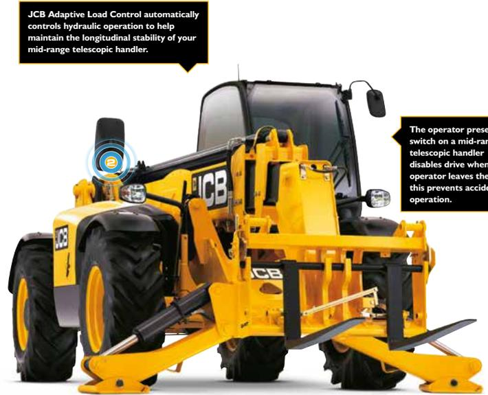
JCB Adaptive Load Control automatically controls hydraulic operation to help maintain the longitudinal stability of your mid-range telescopic handler.
