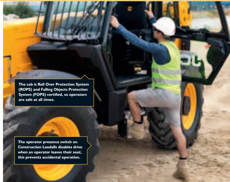
The cab is Roll Over Protection System (ROPS) and Falling Objects Protection System (FOPS) certified, so operators are safe at all times.
