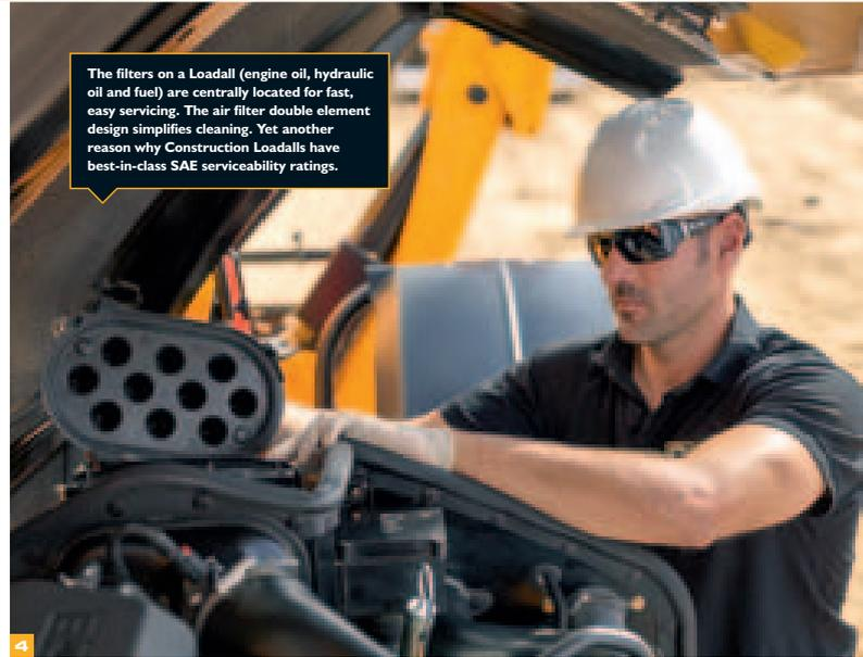
The filters on a Loadall (engine oil, hydraulic oil and fuel) are centrally located for fast, easy servicing. The air filter double element design simplifies cleaning. Yet another reason why Construction Loadalls have best-in-class SAE serviceability ratings.
