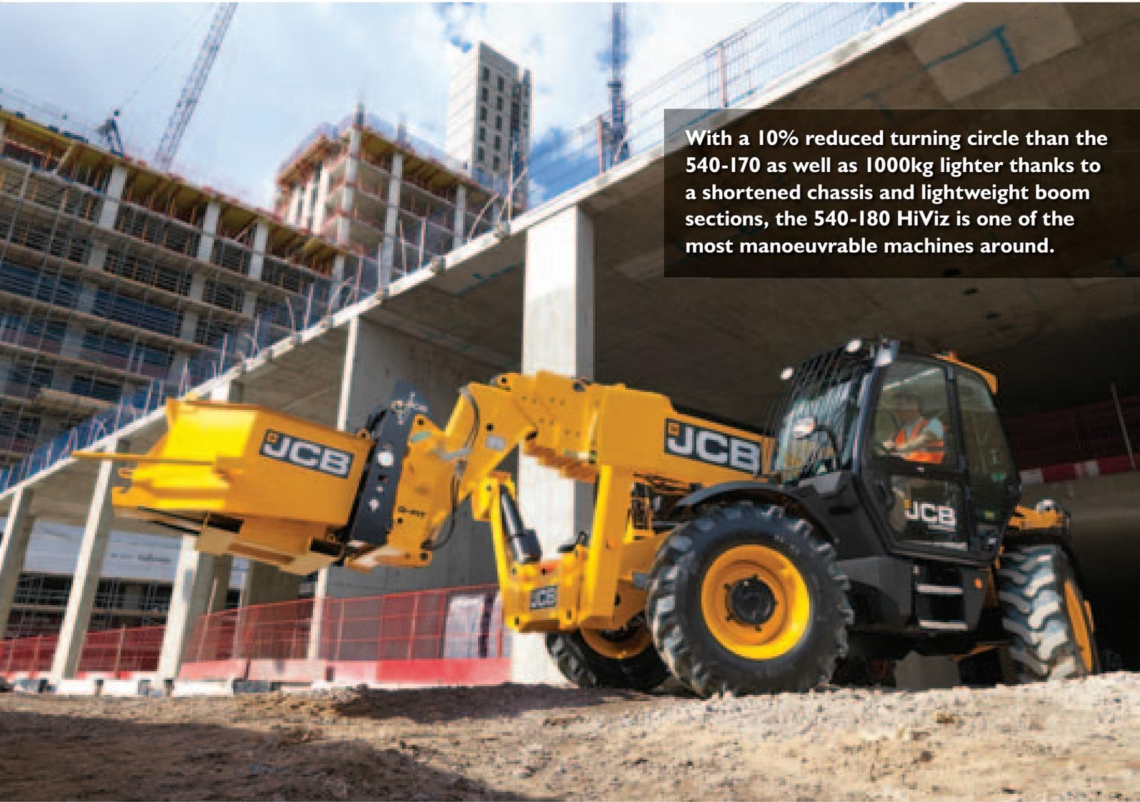
With a 10% reduced turning circle than the 540-170 as well as 1000kg lighter thanks to a shortened chassis and lightweight boom sections, the 540-180 HiViz is one of the most manoeuvrable machines around.
