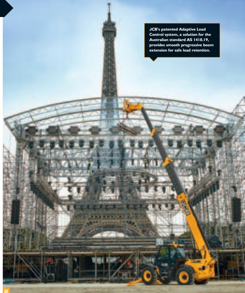
JCB's patented Adaptive Load Control system, a solution for the Australian standard AS 1418.19, provides smooth progressive boom extension for safe load retention.
