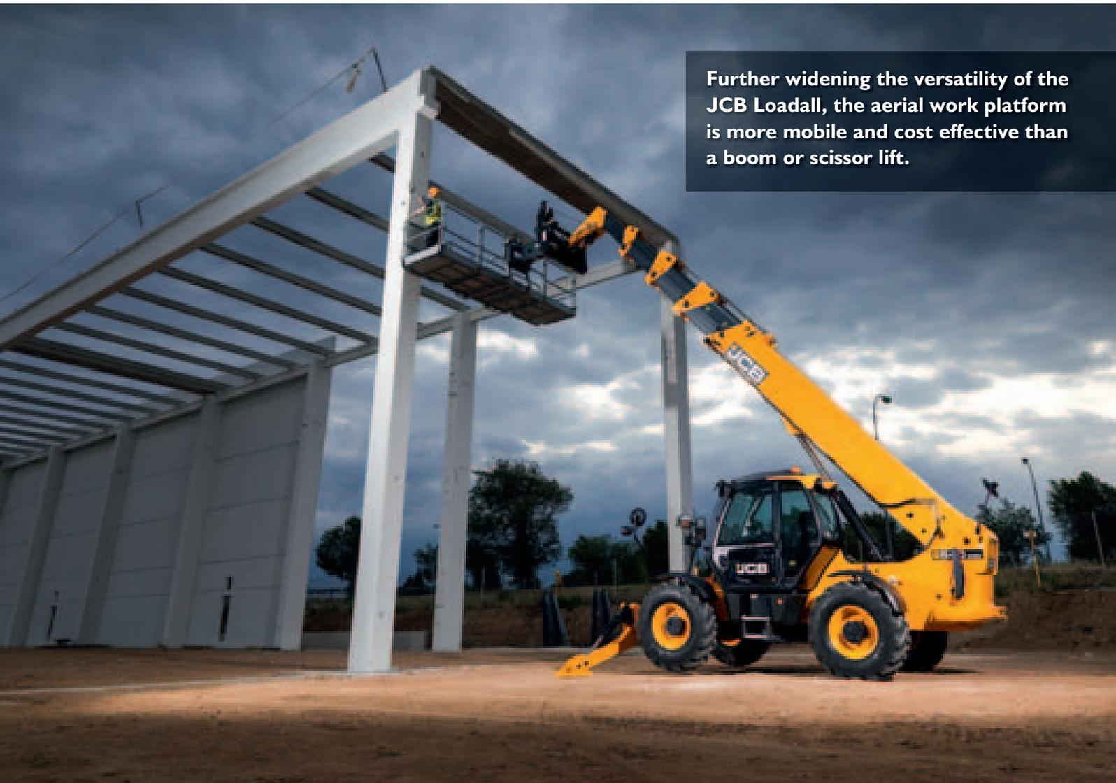
Further widening the versatility of the JCB Loadall, the aerial work platform is more mobile and cost effective than a boom or scissor lift.
