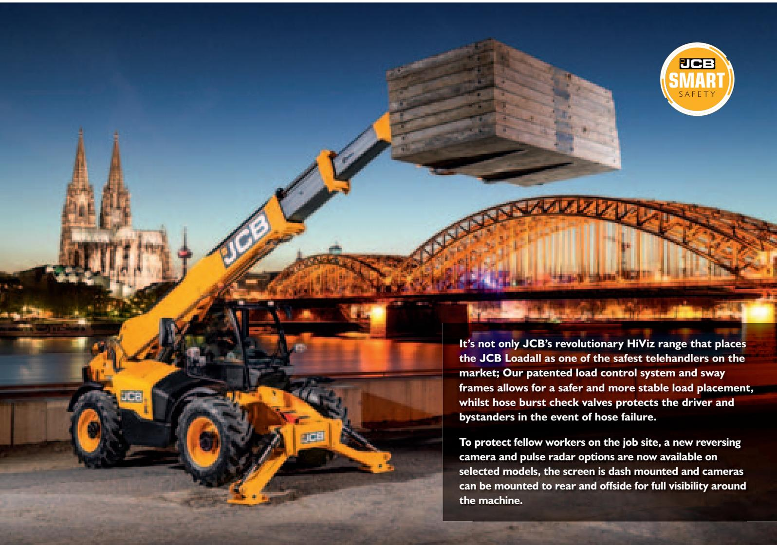
It's not only JCB's revolutionary HiViz range that places the JCB Loadall as one of the safest telehandlers on the market; Our patented load control system and sway frames allows for a safer and more stable load placement, whilst hose burst check valves protects the driver and bystanders in the event of hose failure.
