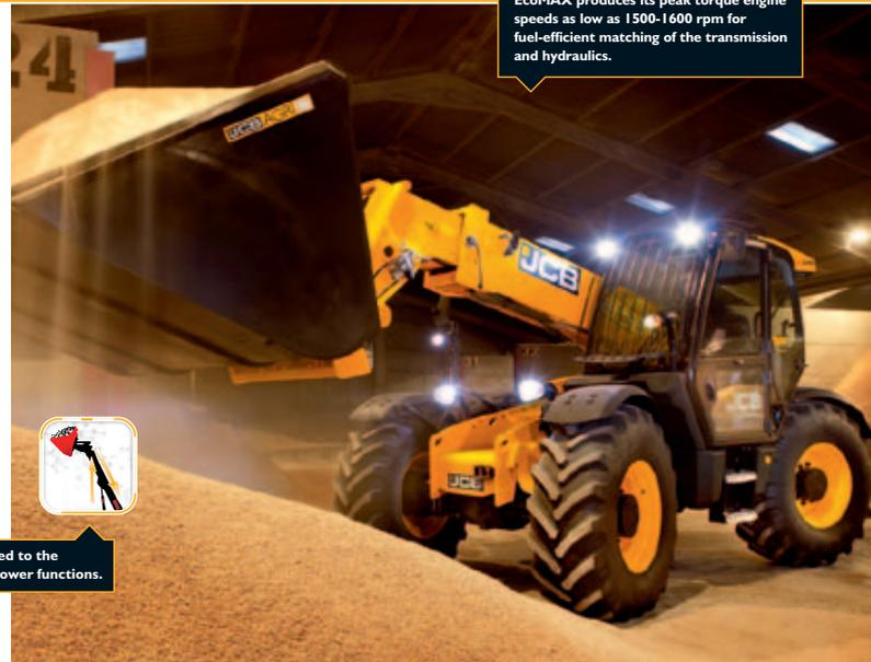
EcoMAX produces its peak torque engine speeds as low as 1500-1600 rpm for fuel-efficient matching of the transmission and hydraulics.
