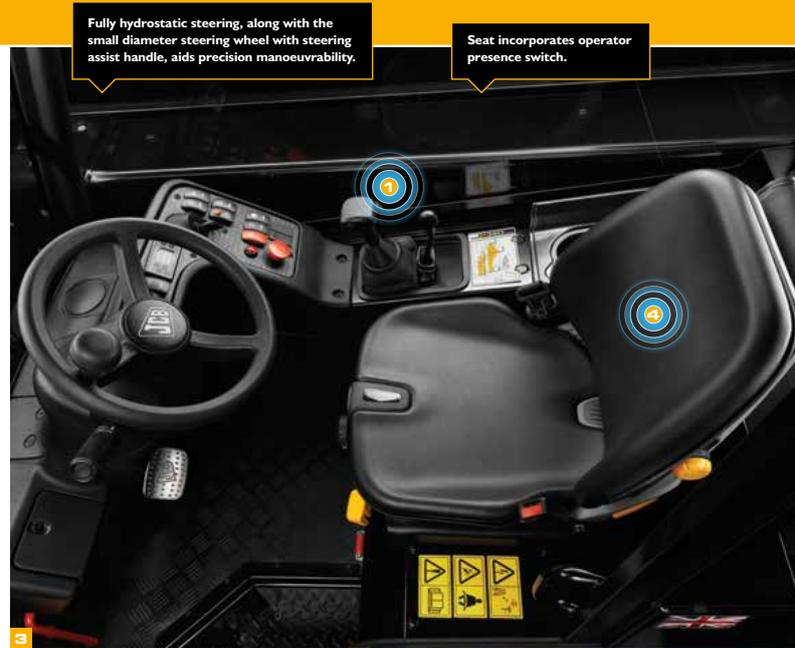
Fully hydrostatic steering, along with the small diameter steering wheel with steering assist handle, aids precision manoeuvrability.
