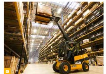
In total, there are ten compact models in the JCB Teletruk range with diesel-powered, fully enclosed hydrostatic drivelines in two and four-wheel drive, and two Gas (LPG) powered two-wheel-drive machines.
