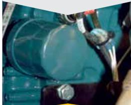
Easily accessible spin on engine oil filter
