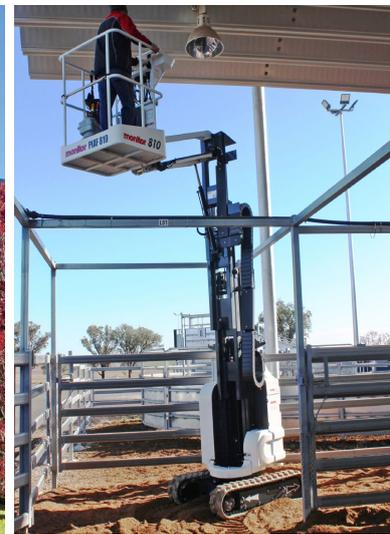
Designed for indoor and outdoor use, these super-compact tracked Mast Lifts are ideal for up-and-over access in very confined areas. The tracks provide excellent stability and traction off-road, and also a soft gentle footprint inside buildings and on other fragile surfaces.
