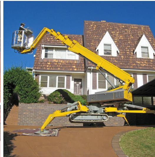
With features including dual power, auto-level, adjustable fly-jib etc, the 23 m Omme Spider Lift weighs only 3250 kg, making it the perfect machine for load-sensitive flooring. The soft non-marking rubber tracks are very gentle on fragile surfaces.
