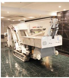
Omme's non-marking tracks are very gentle on sensitive flooring, and the radio-control drive provides ease of manoeuvring in tight areas. With a stowed width of only 1.1 m, the Omme 2750 is perfect for driving down narrow paths and through small gate openings. You will find these Spider Lifts providing solutions to the most difficult access problems in many countries around the world, including Australia and New Zealand!
