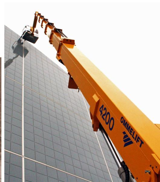
The top of the range Omme 4200 has a huge 42 m working height and a horizontal outreach of 15 m providing an enormous working envelope. And with a weight of only 6.9 t, this Spider Lift is ideal for operating in tight access locations or on load sensitive flooring. The strong all-steel boom sections provide a stable and comfortable platform even at 42 m off the ground!
