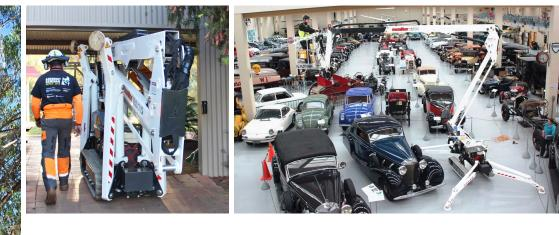
The 1575 is an extremely compact Spider Lift for the most difficult applications. The track system expands out to 1060 mm for extra stability and stands taller for extra ground clearance.
