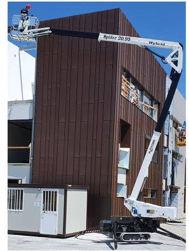
**The newly released 2095 is the best performing Spider Lift that weighs under 3.5 t including a trailer. This means that this machine could be towed behind most tradesmen's vehicles.**
