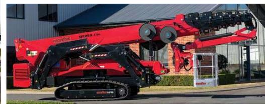
With a massive 43 m of working height, and over 17 m of horizontal outreach, the new 43T Spider Lift is truly a formidable weapon.
