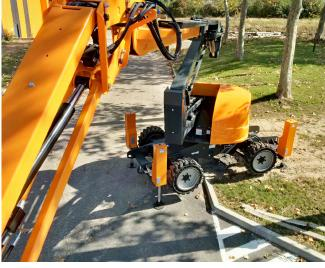
These 4x4 Boom Lifts from ATN are extremely unique in the fact they can be used as a conventional selfpropelled Boom Lift, alternatively the jacks (stabiliser legs) can be deployed from the basket to level the machine on uneven ground. Brilliant? Too right!
